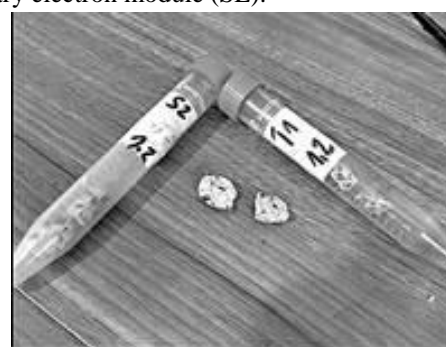
Fig.4: Fragments packaged for porosimetry and microanalysis assay.
