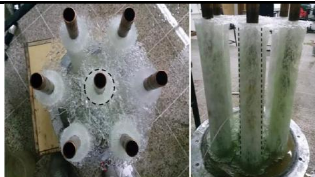
Fig.14: Actual ice thickness in the storage tank.
