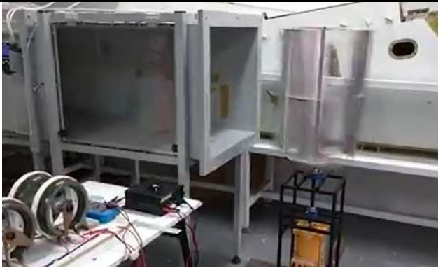
Fig. 9: Lenz-type turbine under tests.
