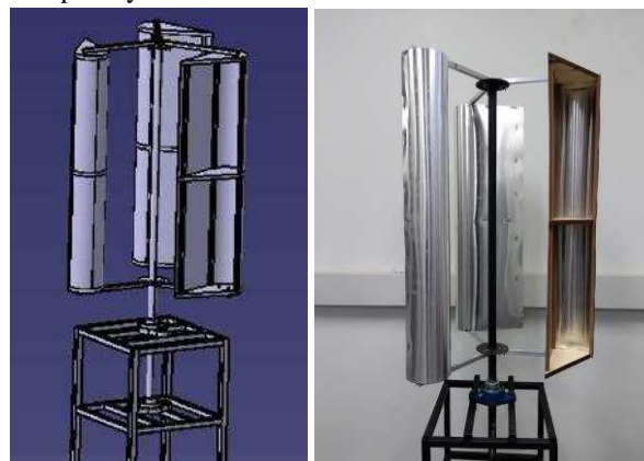
Fig. 8: 3D-drawing and photo of the Lenz-type VAWT.
