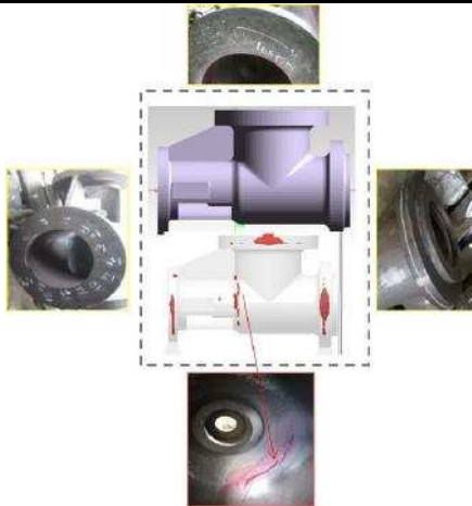
Fig.5: NDT-UT Product vs Magmasoft Comparison
