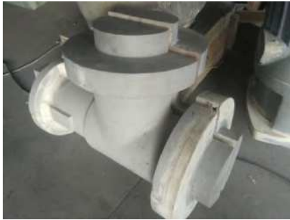
Fig.11: Wooden pattern middle part ESV
