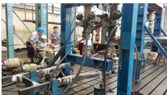
Fig.12: Bending test on bent chassis
