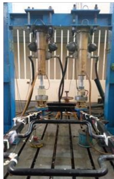
Fig.15: Torque test on welded chassis
