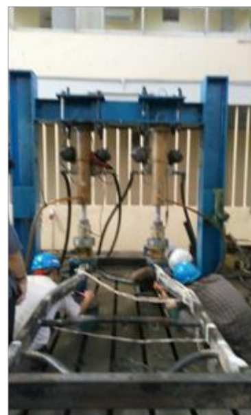
Fig.16: Torque test on bent chassis
