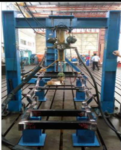
Fig.11: Bending test on welded chassis
