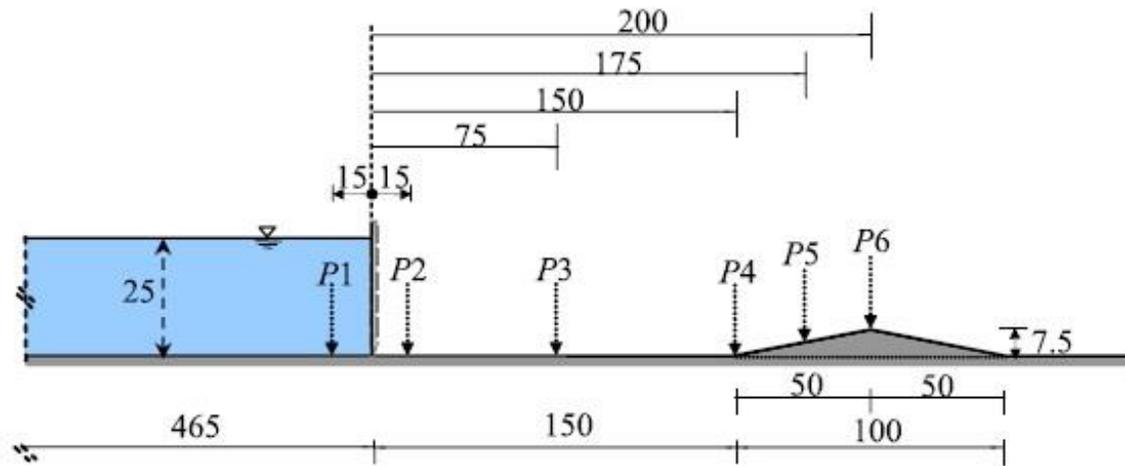
Fig.2: The measurement locations of the stage hydrographs, lengths in [cm] [14]
