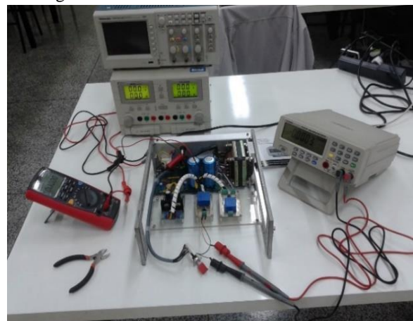
Fig. 3: Calibration experiment for the voltage sensor.
