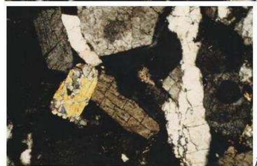
Fig. 12-13: Observation of thin blade of the beige vosgian sandstone before (12) and after (13) treatment with pH 12.6
