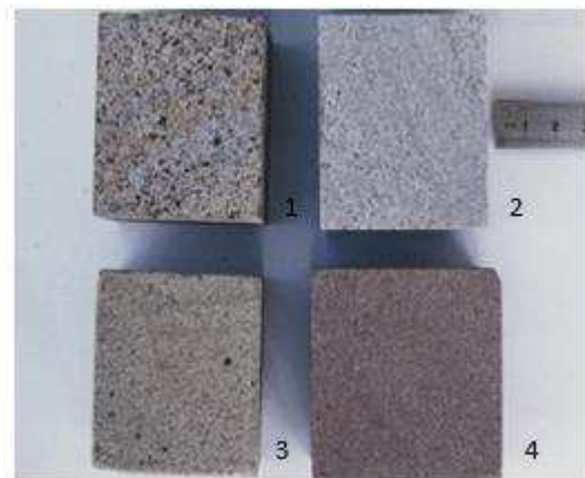
Fig. 1: Macroscopic aspect of sandstone materials, reflecting the differences in mineralogical composition and matrix that gives the rocks their specific color, 1- molière sandstone, 2-coal sandstone, 3- beige vosgian sandstone, 4- red vosgian sandstone.
