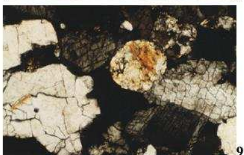
Fig. 8-9: Observation of thin blade of the red vosgian sandstone before (8) and after (9) treatment with pH 12.6
