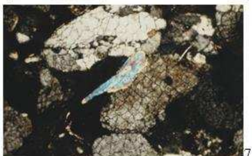
Fig.6-7: Observation of thin blade of the coal sandstone before (6) and after (7) treatment with pH 12.6
