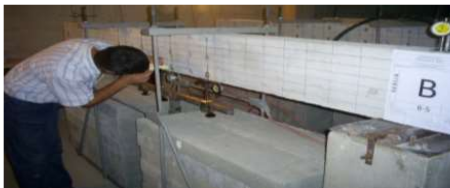
Fig.2: Measurement of the crack with and gravitationally load from concrete cerbs [3].
