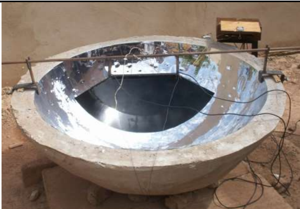
Fig.14: Image of the prototype - Concrete hemispherical concentrator with it moon crescent-like absorber.
