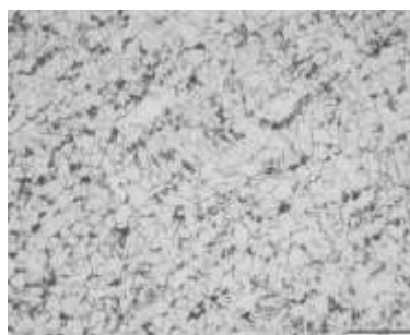
Fig.10: Microstructure of re-heat refined zone in weld deposit due to GTAW + HF dressing
