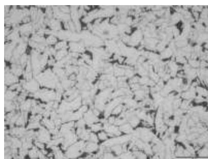
Fig.16: Microstructure of re-heat refined zone in weld deposit due to P-GTAW + HF dressing
