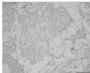
Fig.9: Microstructure of dressed weld deposit by conventional GTAW + HF
