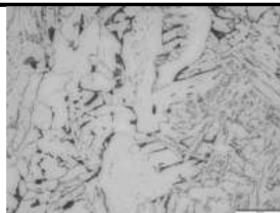
Fig.15: Microstructure of dressed weld deposit by P-GTAW + HF
