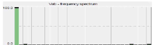
Fig.14: Frequency Spectrum for Vab during mitigation of L-L fault
