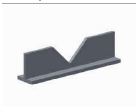
Fig: 3 Fins with V – Shaped Notch
