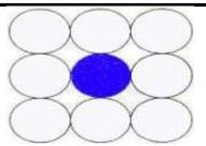
The 4-connected pixel technique failed to fill the area as marked in the following figure which won't happen with the 8-connected technique.
