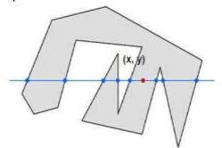
From the above figure, we can see that from the point (x,y), the number of interactions point on the left side is 5 and on the right side is 3. From both ends, the number of interaction points is odd, so the point is considered within the object. [2]
