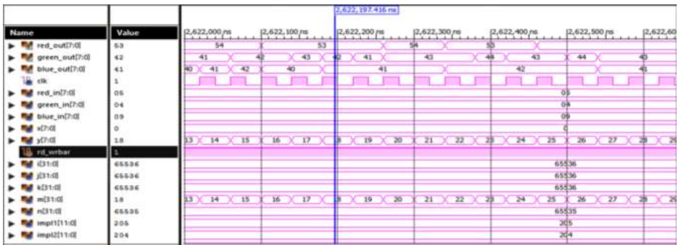
Fig. 7(b). Waveform of RGB Pixels when read write bar = 1
