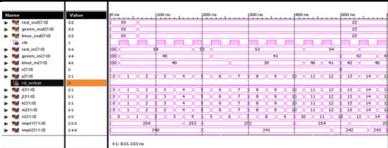
Fig. 7(a): Waveform of RGB Pixels when read write bar = 0
