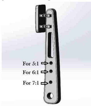
Fig 2:-Holes for variable pedal ratios
