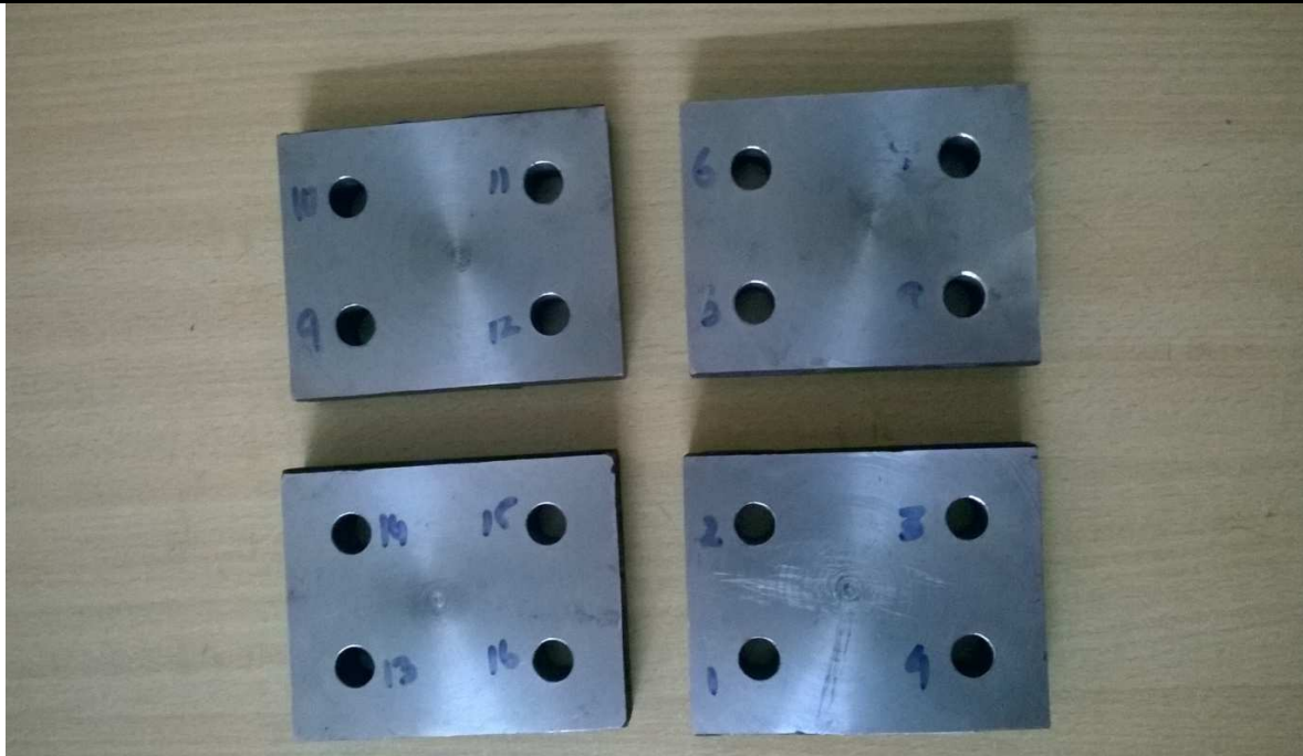
Fig.2: H13steel drilled specimen ( L_{16} )
