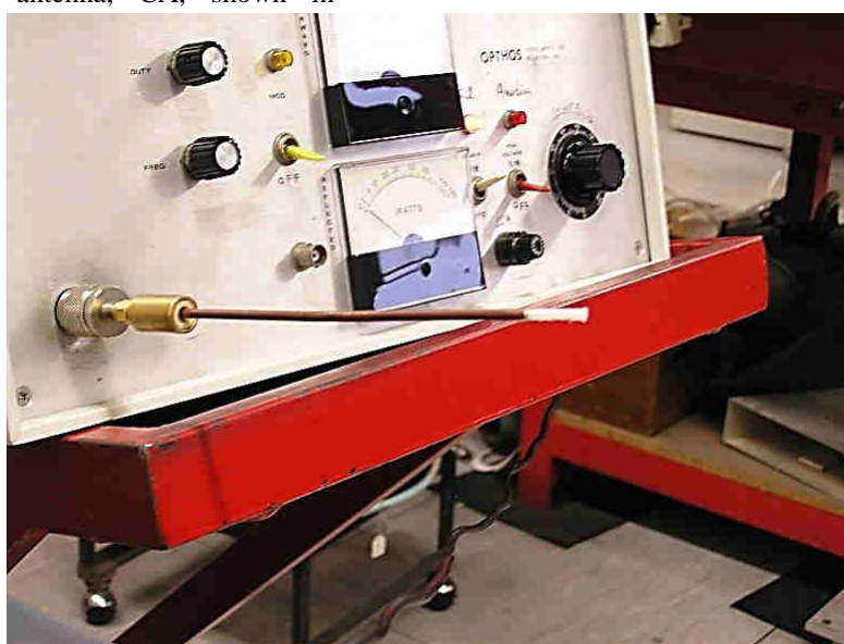
Fig. 2: Coaxial dipole antenna attached to the output port of microwave source. The dielectric-tip end is evident in the foreground.
