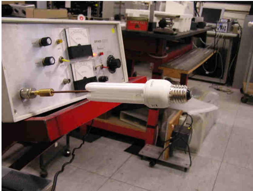
Fig. 3: The dipole antenna is placed along the axis of the fluorescent lamp.
