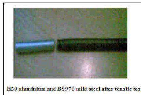
Fig.4: H30 aluminium and BS970 mild steel after tensile test
