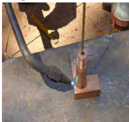
Fig. 2.3: Brazing of tool Fig. 2.4: Bottom of tool
