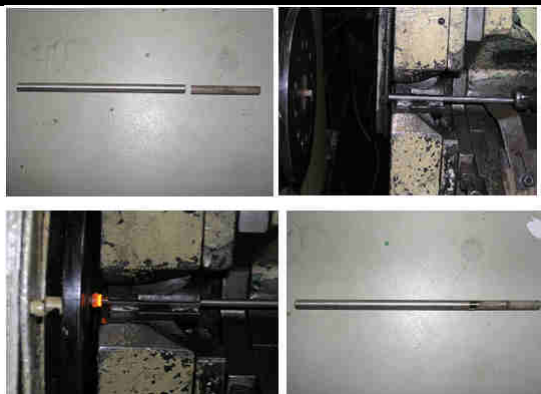
Fig.2 : Friction Welding Operation In “Pin To Pin” Process
