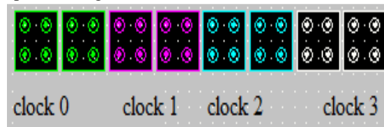
Fig.6.QCA cell four clock zones
