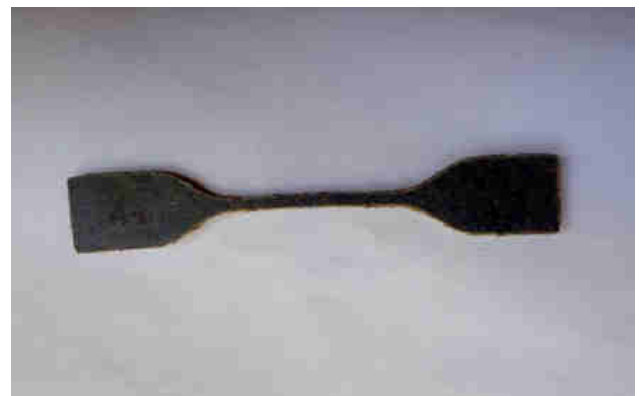
Fig. 3: Specimen for tensile test
