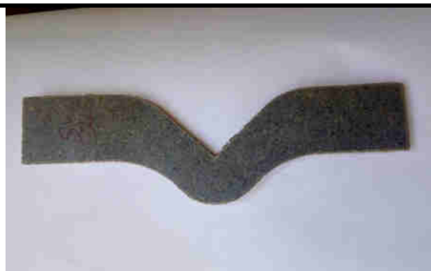
Fig. 6: Specimen for tear test
