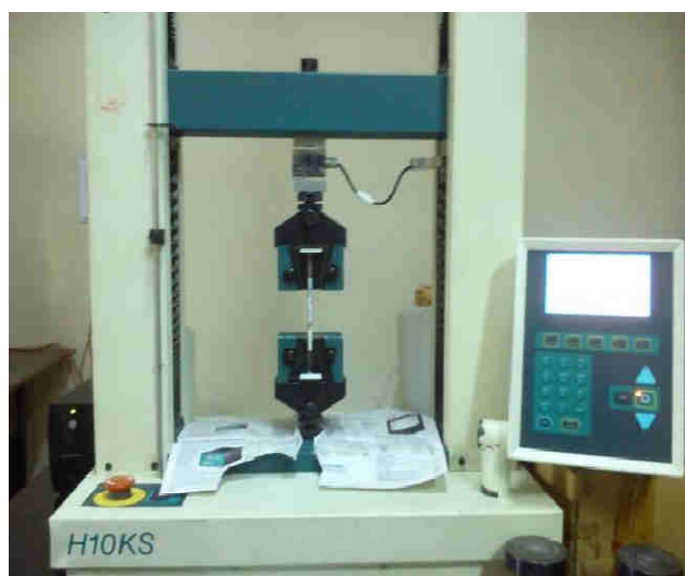
Fig .3: Loading arrangement of tensile test
