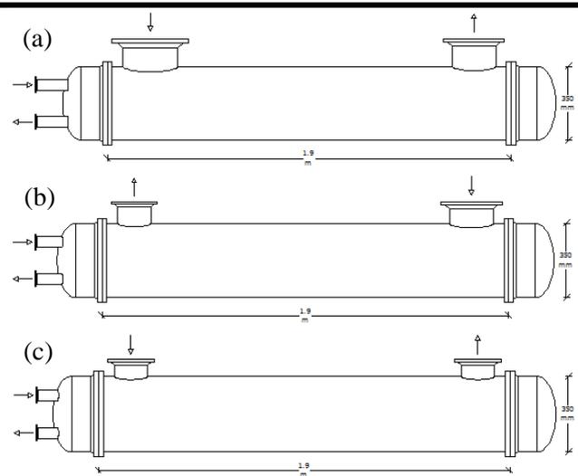
Fig.3: Sketch layout of 1<sup>st</sup> intercooler (a), 2<sup>nd</sup> intercooler (b), and aftercooler (c)
