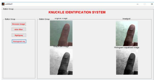
Fig. 5: Pre-processing of finger knuckle image
