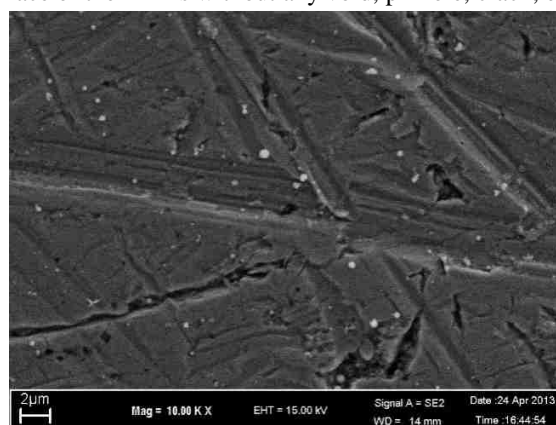
Fig.2:FESEM Photograph of as deposited CdS film
