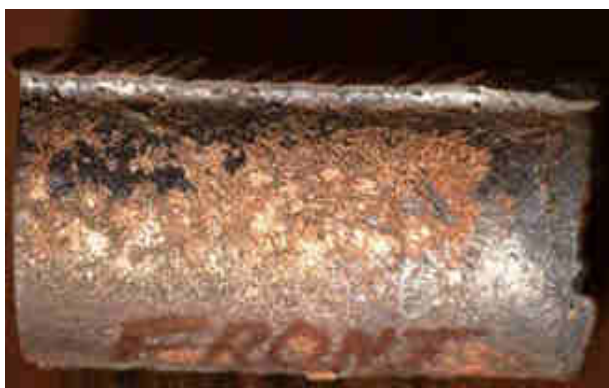
Fig.3.1: Water wall tube before failure tube
