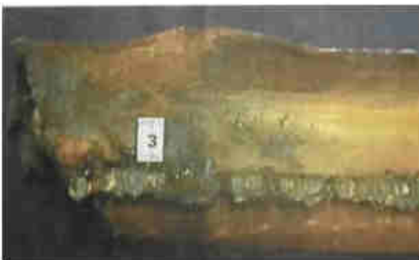
Fig.3.3: External metal wastage
