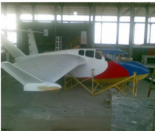
Figure 14 The WISE craft 8 seaters Lippisch configuration prototype B type.
