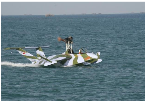
Figure 9 The WISE-craft 2 seaters A2B prototype flight tested on the sea.
