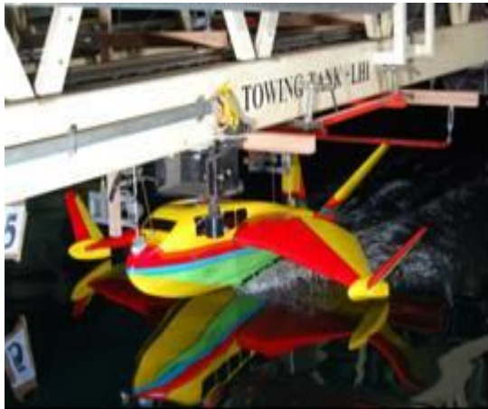
Figure 8 Towing tank test model in the IHL, Surabaya.
