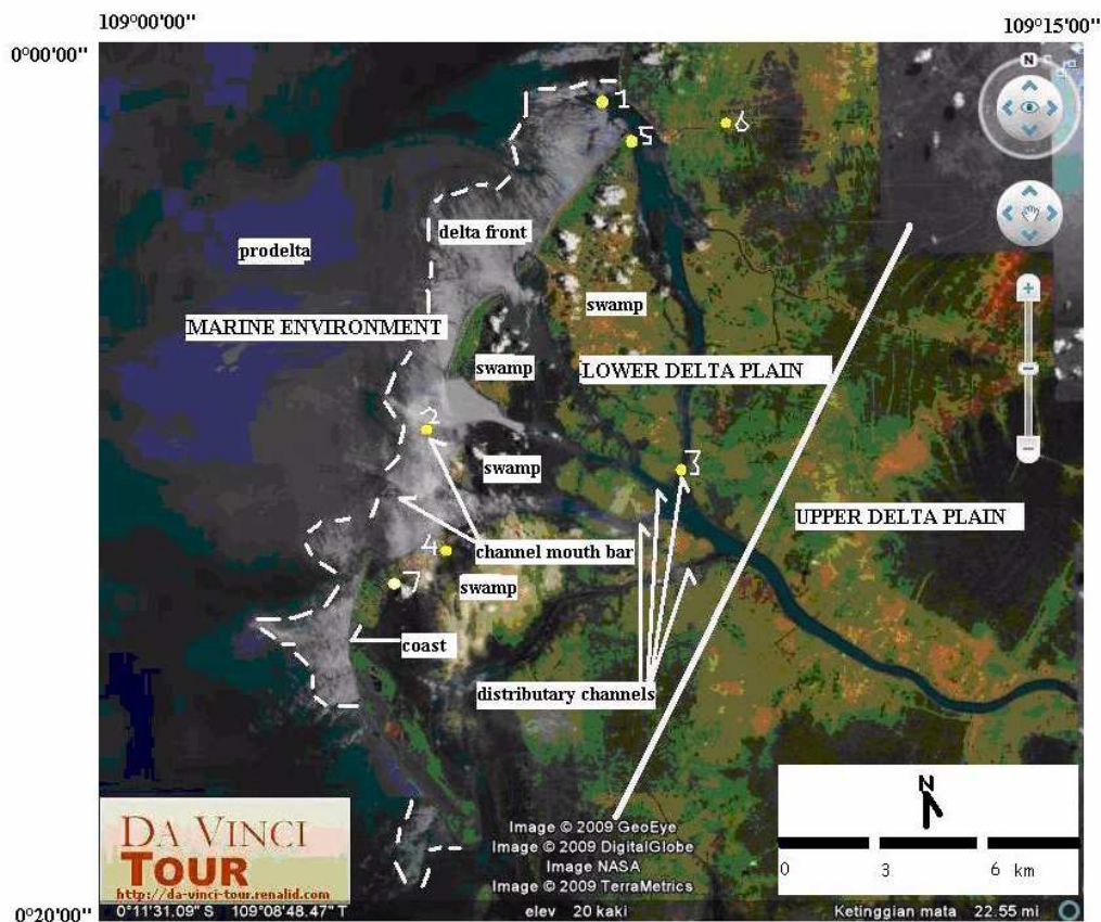
Figure 2. Recent deltaic deposition environment of the Kapuas Delta (from earthgoogle satellite imagery). Marine environment consist of prodelta, delta front and channel mouth bar; while lower delta plain composed of deltaic islands, distributary channels, swamp and coast. Upper delta plain was not discussed due to not located in coastal zone. Numbers are drilling locations.
