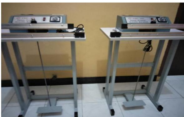
Gambar 5. Mesin Sealer Model Pedal
