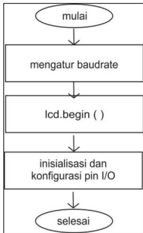
Gambar 2. Diagram alir prosedur setup()
