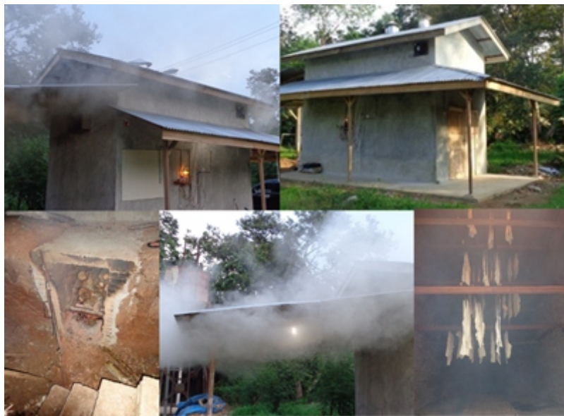
Gambar 3. Pengujian ruang kendali temperatur asap RSS Figure 3. Experiment smoke temperature control for RSS
