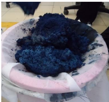
Figure 6. Sample of indigo paste produced from aeration experiments
