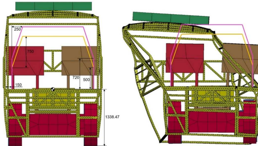
Figure 12 Fully loaded bus residual space envelope before and after rollover test.
