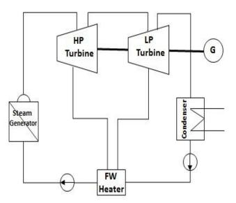
Fig. 1 The internal nuclear power plant cycle.
