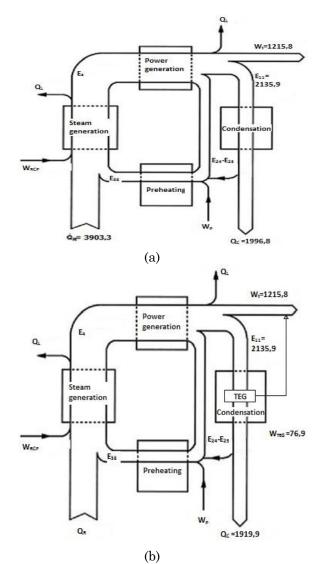
**Fig. 6.** (a) The simplified balance diagram for energy (in the units of MW) and (b) The simplified energy balance diagram with the installed prototype TEG unit of NPP.
