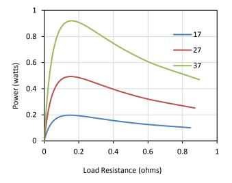
Fig. 8. HZ-20 Manufacturer characteristics datasheet for the power outputs with the load resistance in the cases of  $\Delta$ T=17,  $\Delta$ T=27 and  $\Delta$ T=37°C.
