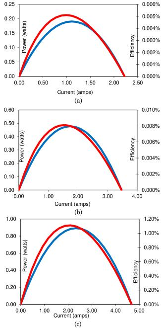
Fig. 7. HZ-20 Manufacturer characteristics datasheet for the power outputs (blue) and efficiencies (red) with respect to electric current in the cases of (a)  $\Delta$ T=17, (b)  $\Delta$ T=27 and (c)  $\Delta$ T=37.
