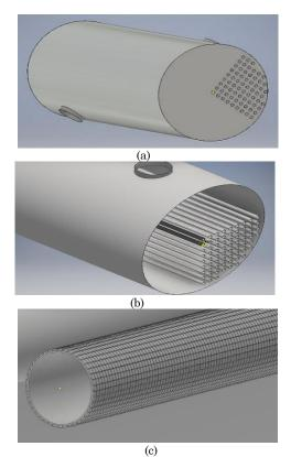
**Fig. 3** (a) The inside view of the revised TEG prototype of condenser, (b) The schematic representation of arrangement of TE modules inside of the condenser, (c) The covered with thermoelectric modules design for the tube.
