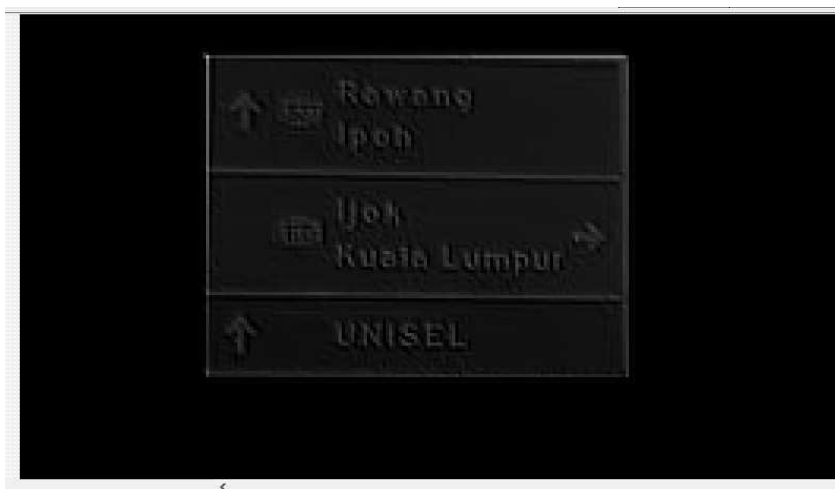
Figure 5 Image after edge detection.
