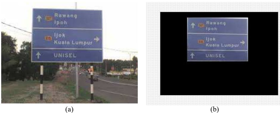
Figure 3 (a) Image before ROI is performed, (b) image after ROI is performed.
