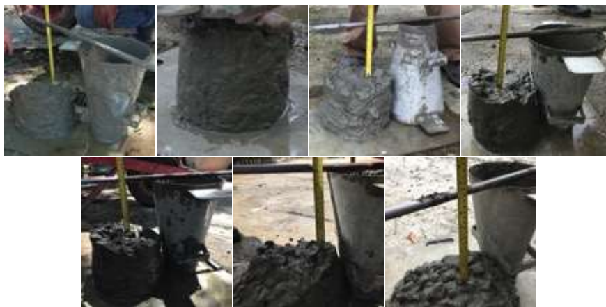
Figure 1. Concrete slump: from right to left A 0 , A 1 , B 1 , C 1 concrete ( up row ), A 2 , B 2 , C 2 concrete ( bottom row )
