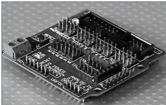
Gambar 12 *Shield I/O* Sebelum Dipasang Header Male
