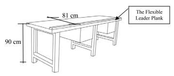
Figure 5 Redesain the Working Table for Fabrication
