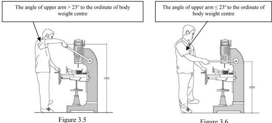
The Angel of the Handle of Drilling Bit and the Work Posture Before Redesign Work Station
