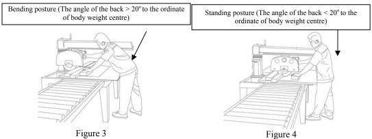
The Work Posture at the Radial Saw Machine before Redesign Work Station
