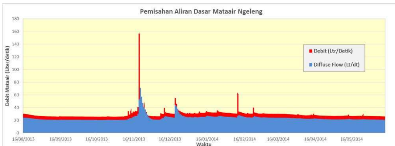
Gambar 6. Hasil Automated Baseflow Separation by Digital Filtering Mataair Ngeleng. (Sumber: Olah data primer, 2014)
