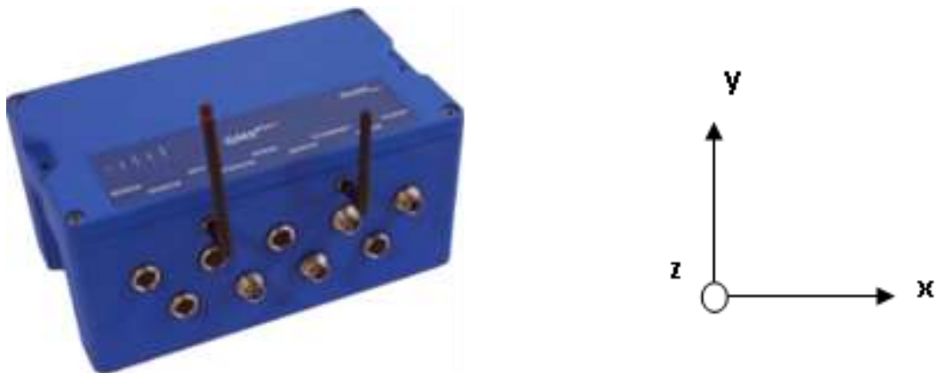
Figure 4. GeoSig accelerometer and its direction
