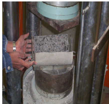
Figure 2. Splitting of specimen under tension
