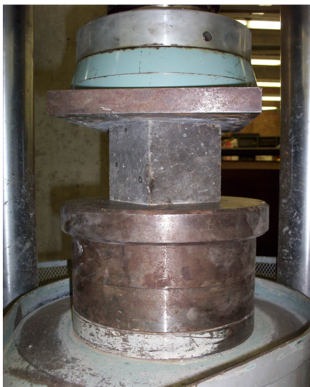
Figure 1. Compressive strength test
