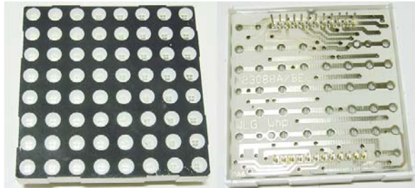
Gambar 10. Gambaran Fisik LED-Matrix Pack M23088A
