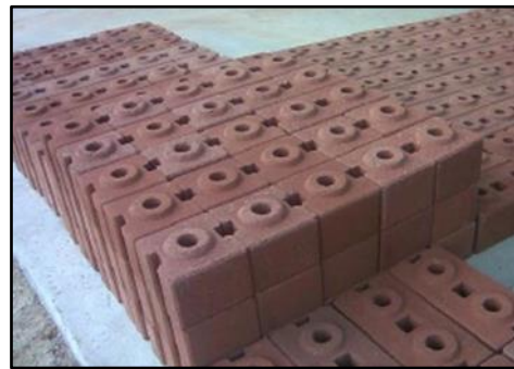
Gambar 1. Soil-Cement interlocking block Sumber: Masha Chavoshi, 2011
