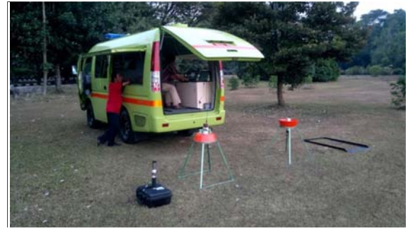
Fig. 4. Outdoor air measurement of ^{131}\text{I} by direct method.
