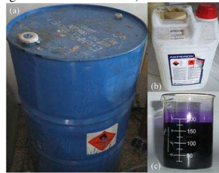
Gambar 4. Material matriks fiberglass (a) Vynil Ester Resin (b) katalis (c) Cobalt
