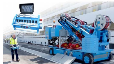
Figure 4. Cable management system using robot arm by Stemmann Technik
