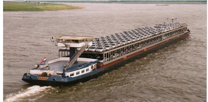
Gambar. 2. Self-Propelled Car Barge di sungai Rhine, Jerman [5]
