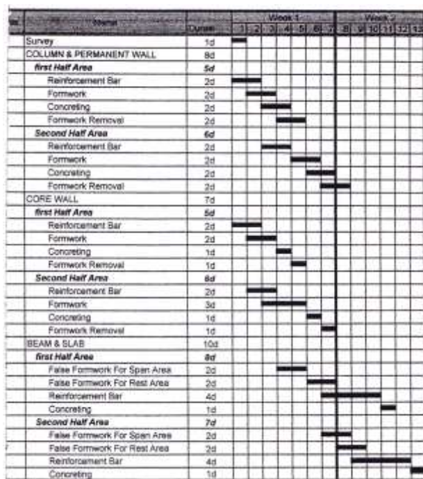
Gambar 4.6 Schedule For Typical Floor
